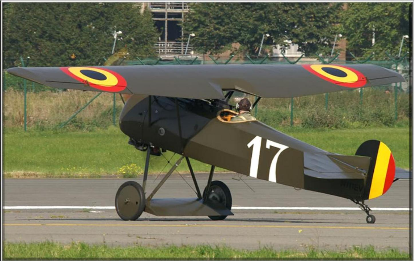
The **Fokker E.V** was a [German parasol](#)-monoplane [fighter aircraft](#) designed by Reinhold Platz and built by [Fokker-Flugzeugwerke](#). It entered service with the [Luftstreitkräfte](#) in the last months of [World War I](#). After several fatal accidents due to wing failures, the aircraft was modified and redesignated **Fokker D.VIII**. Dubbed the *Flying Razor* by Allied pilots, the D.VIII had the distinction of scoring the last aerial victory of the war.
