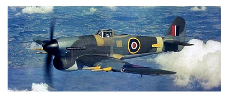
The **Hawker Typhoon** was a British single-seat <u>fighter-bomber</u>, produced by <u>Hawker Aircraft</u>. While the Typhoon was designed to be a medium-high altitude <u>interceptor</u>, and a direct replacement for the <u>Hawker Hurricane</u>, several design problems were encountered, and the Typhoon never completely satisfied this requirement. Other external events in 1940 prolonged the gestation of the Typhoon.
