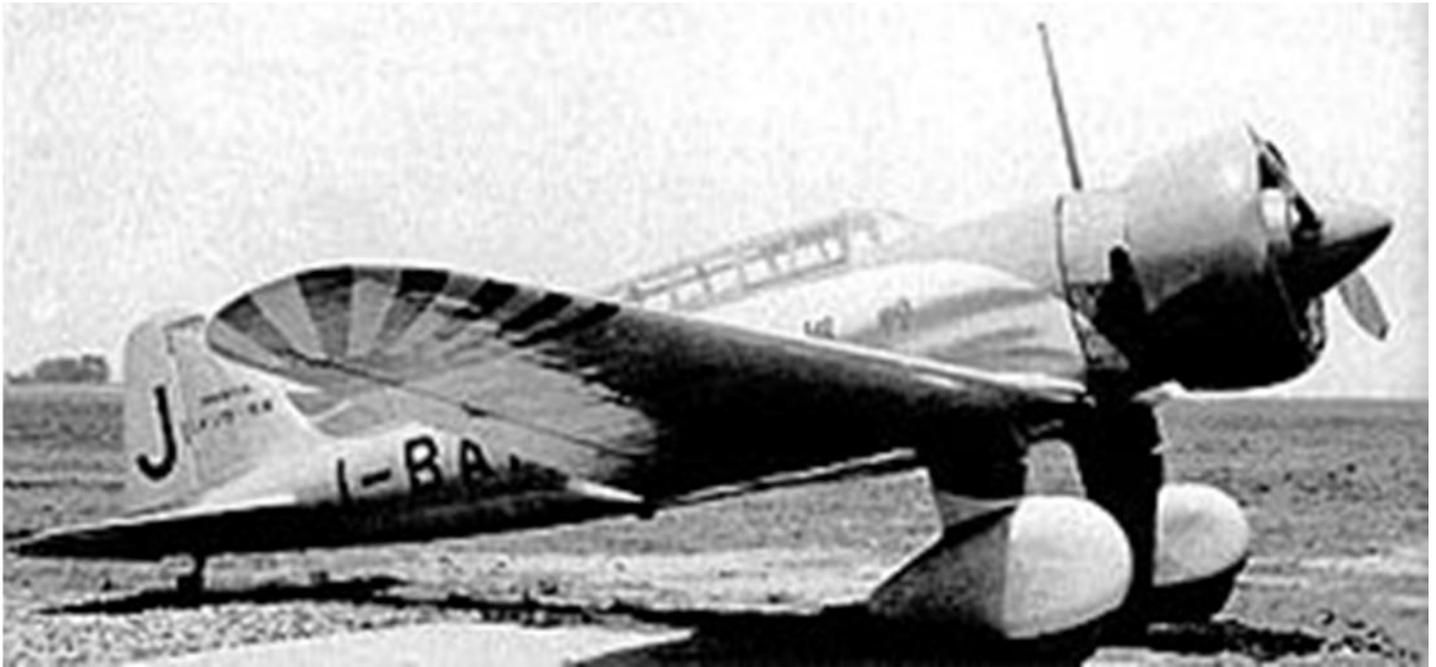
Plans were already in hand to improve the Ki-15-I, and in September 1939 the **Ki-15-II** was put into production with the 671 kW (900 hp) [Mitsubishi Ha-26-1](#); the smaller diameter of this both reduced drag and overcame one of the major shortcomings of the initial version: poor forward field of view past the large-diameter of the initial [Nakajima Kotobuki](#) engine. The improved version entered production in September 1939 as the Ki-15-II.
