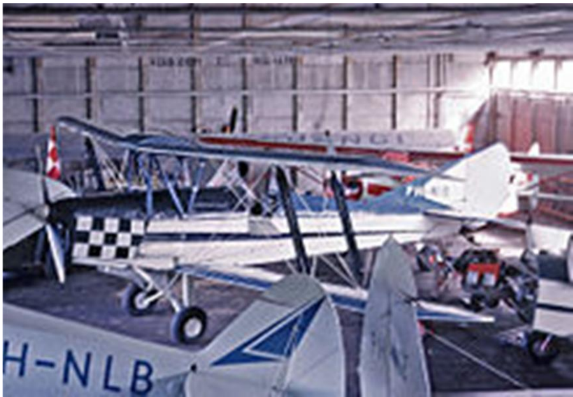
Dutch Tiger Moth with the extended fin area required by the local authorities
